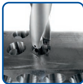
Vollbohren Solid drilling
